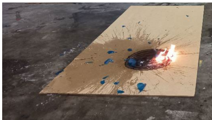
Figure 9: The result of test 11, the fire wasn't completely extinguished
