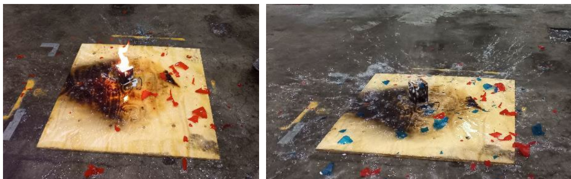
Figure 16: The result after throwing the first Flame Away (left) and after throwing the second Flame Away (right)
