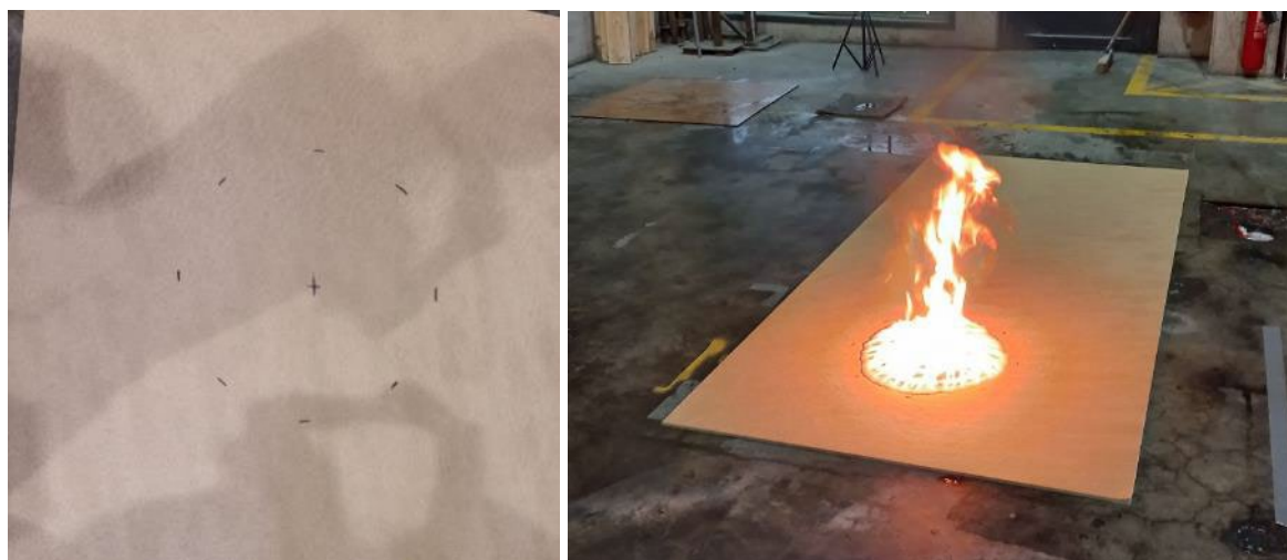
Figure 2: The outlined circle in which the kerosene was spread (left) and after the kerosene was set on fire (right) on the softboard.
