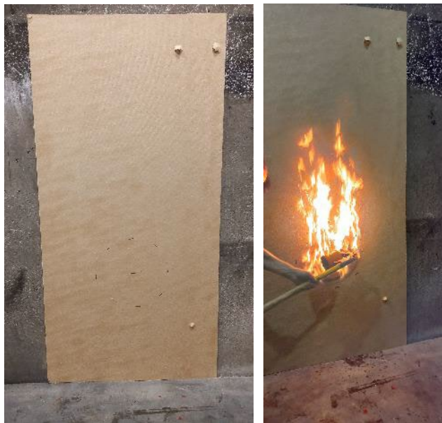
Figure 5: The vertical softboard wall with the outlined circle in which the kerosene was spread (left) and set on fire (right)
